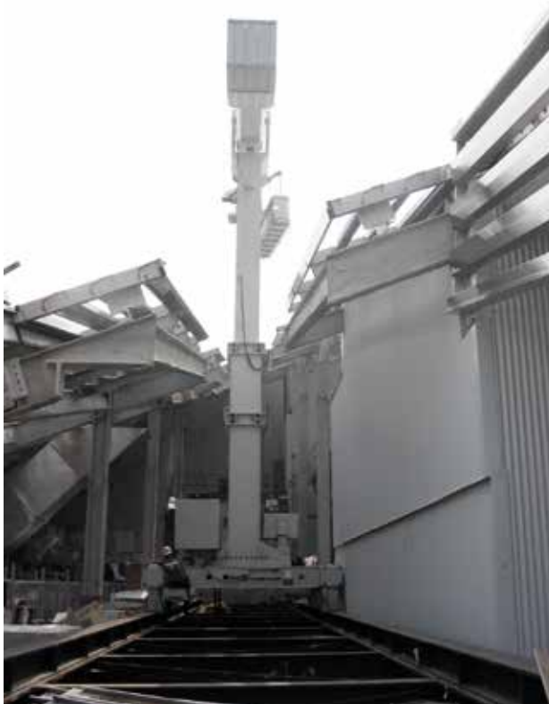
Hydraulically operated telescopic slewing mast
