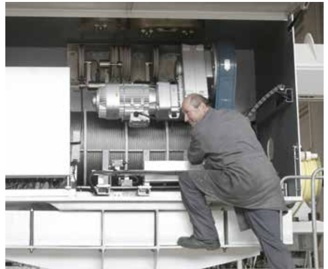
► High-performance hoist unit, approx. 4,000kg lifting capacity.
