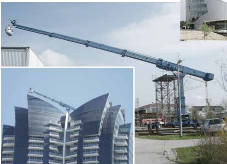
Type 6.4 with a quadruple telescopic jib, slewing device and telescopic mast. Unit assembled at factory for testing and mounted on building roof.
